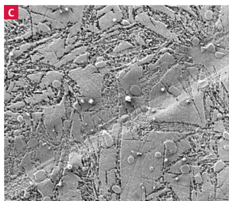
Figure 5 (C): BSE image of the same location on the steel sample. The image is formed by collecting electrons traveling closer to the sample surface.
