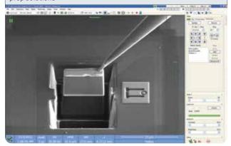
↑ Control of the EasyLift is integrated into the DualBeam UI. Movement of the probe can be done on screen with the mouse.
