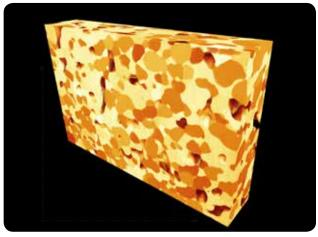
↑ Offline reconstruction of 3D volumes. Reconstructed 3D volume of a fuel cell electrode using ResolveRT\*. Sample courtesy of Sabanci University, Turkey.
