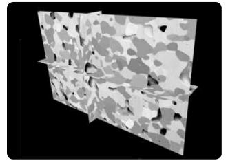
↑ Orthoslices of the fuel cell electrode. With ResolveRT, the slices can be moved through the sample exhibiting details in the 3D volume. Movies can be created that display the movements through the sample.
