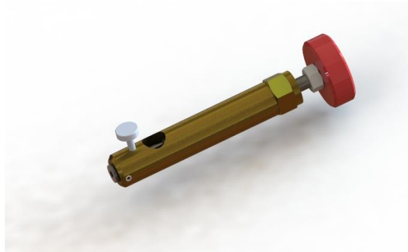
Figure 5-4. Carbon rod shaper (red handle) for preparing 1.4mm (dia) spigot
