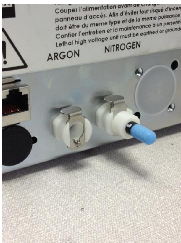
Figure 2-2. Gas connectors with filter (part no. 12842) fitted to purge gas inlet
