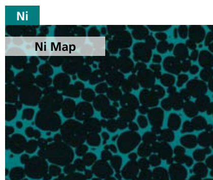
EBSD Phase map and X-ray spectral images acquired from an alloy of tungsten particles in a nickel matrix. Simultaneous data acquisition was at 870 points per second, indexing hit rate was 99%. Using NordlysMax 2 and X-Max data acquisition is possible in minutes.
