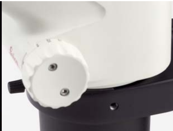
8:1 zoom with 2 adjustable zoom stops for repetitive tasks
