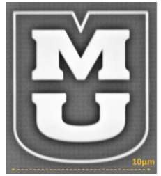
Left: Large-scale cross-section generation to confirm oxide layer thickness (courtesy H. Wen) Right: Patterned microdeposition of W+C with ~200nm resolution (EMC staff)
