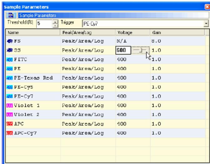
Figure 3.15 Set Gain for the Voltage
