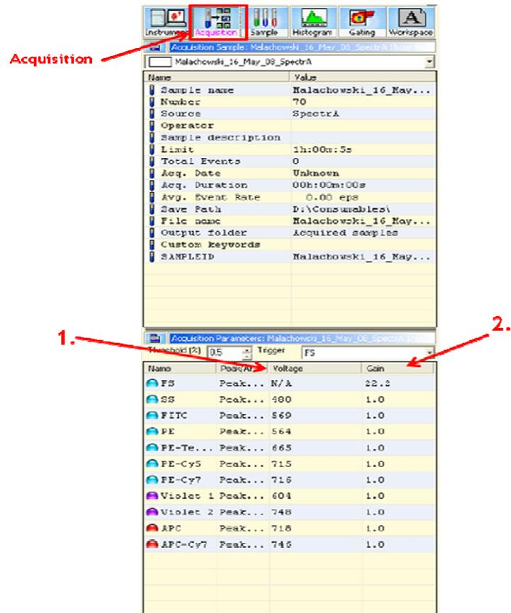
Figure 3.14 Set Voltage for a Parameter
