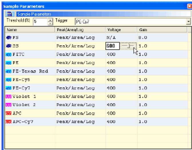
Figure 3.15 Set Gain for the Voltage
