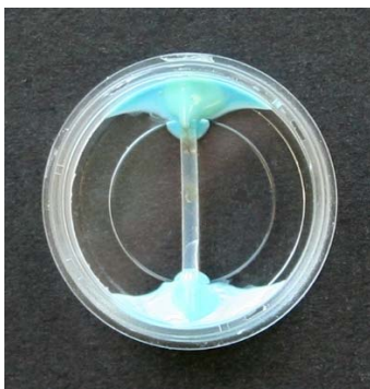
Figure 2. Sample preparation using FEP tubing and Twinseal.
