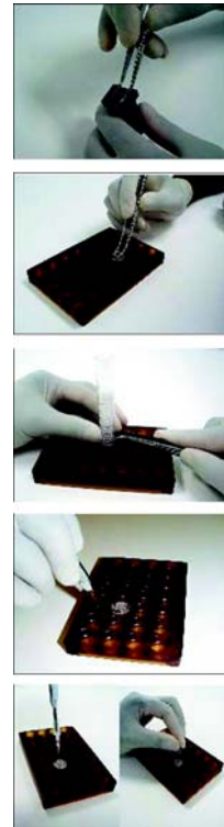
Figure 8.2: Placing assembled CapSure HS Cap and Extracsure Device in the Alignment Tray.
